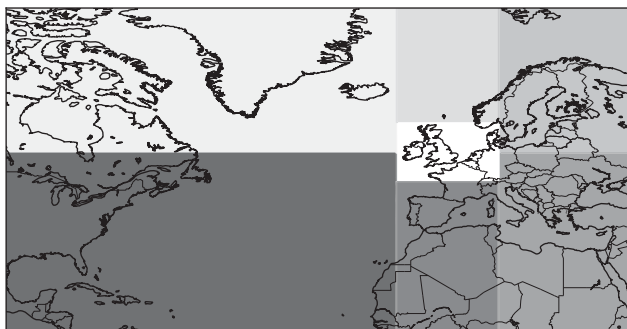
Figure 6. Schematic of the arrangement of the full NAME computational domain, divided into six fixed regions and the sub-domain in which the transdimensional inference was performed, shown by the different shadings.
