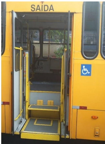
Photograph 7. Bus lift in Curitiba
