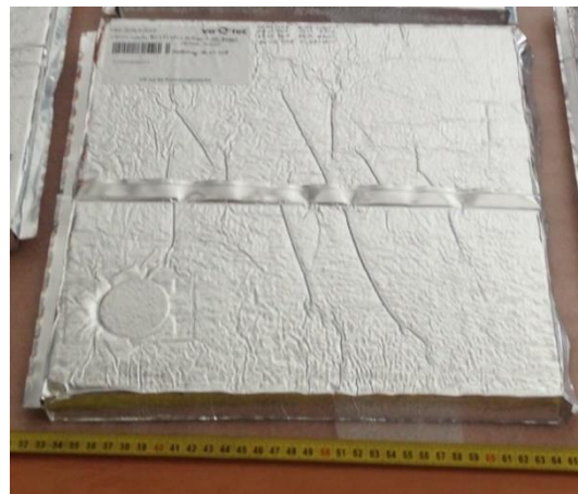
Figure 11: VIP made from new polymeric foam.
