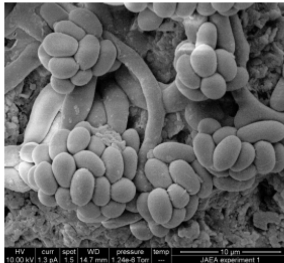
Figure 9 CryoSEM SEI image of the fracture surface showing detail of clusters of rod-like cells associated with biofilaments. Post-experimental material (Biotic Experiment). High vacuum cryoSEM, uncoated sample, FEI ESEM instrument.
