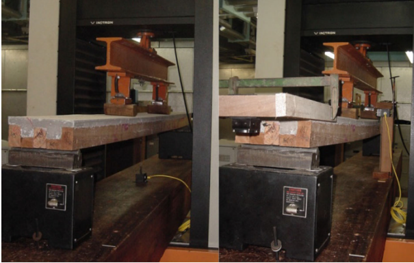
Fig. 4 Wood–concrete beam test specimens for set 1.
