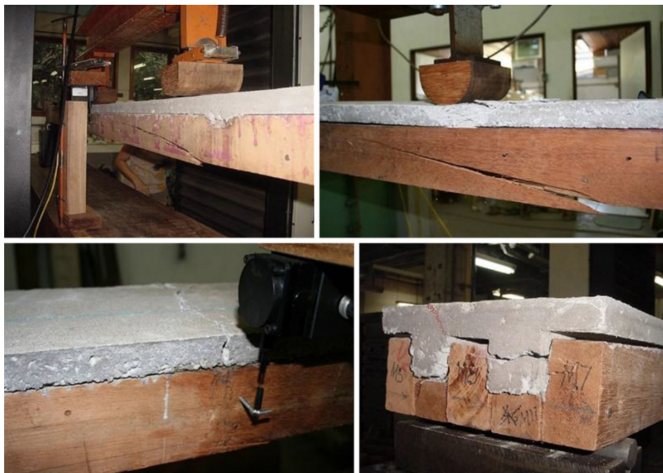
Fig. 6 Tensile failure in the wood and shearing of the concrete.
