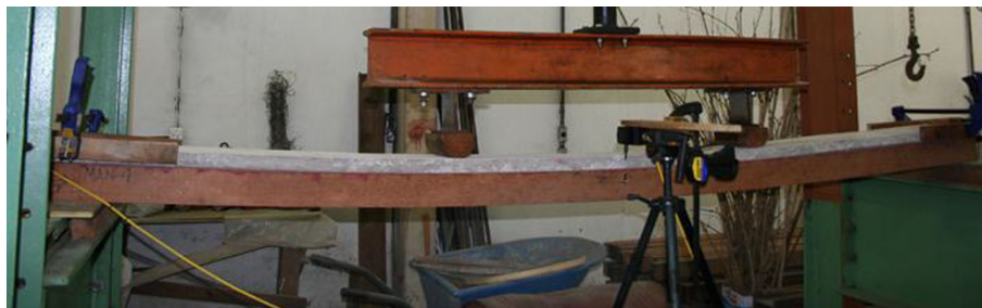
Fig. 5 Wood–concrete beam tested on third-point loading for set 2.
