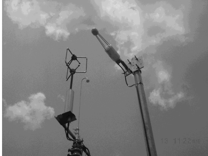
Fig.2: Fast response instruments in the meteorological tower at Rebio-Jarú.
