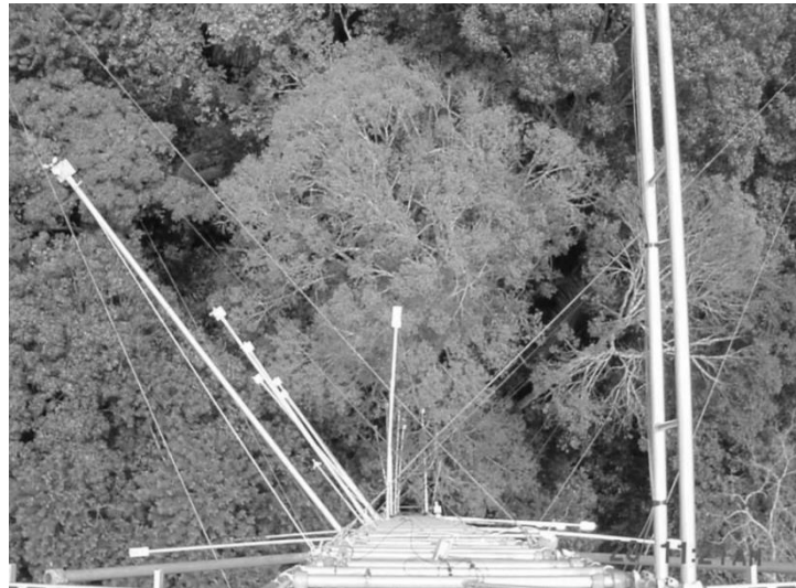
Fig. 3: Cup anemometers ranged at different heights in the meteorological tower at Rebio-Jarú
