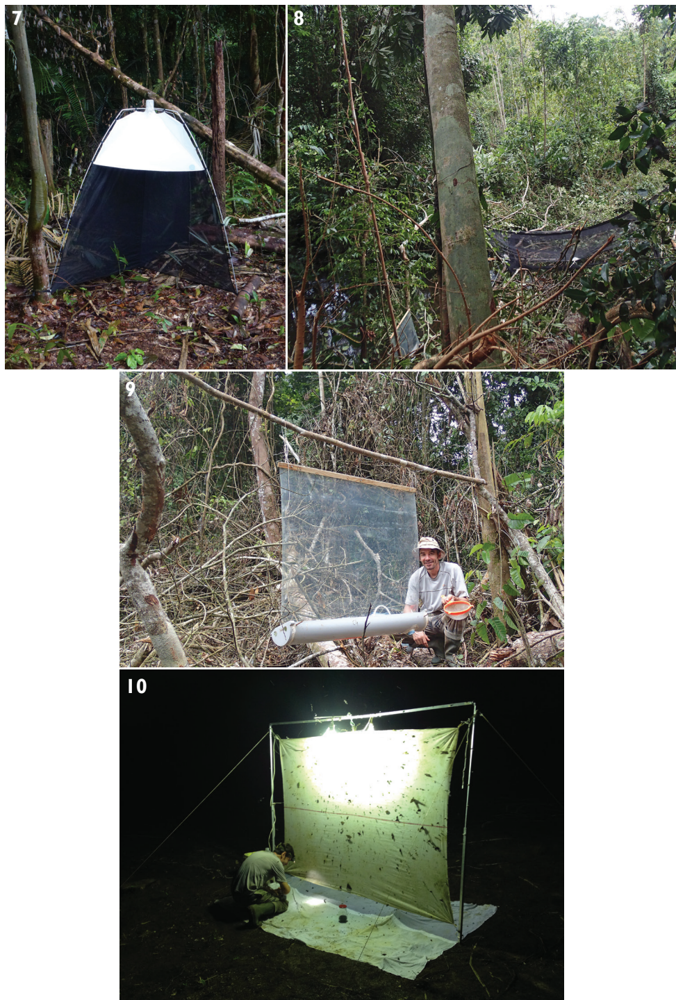
Figures 7–10. Collecting techniques applied during Mitaraka survey 7 SLAM (photo Marc Pollet), 8 6m long Malaise trap (MT) (photo Julien Touroult) 9 flight intercept trap (FIT), with Eddy Poirier (photo Julien Touroult) 10 light trap (LT), with Eddy Poirier (photo Marc Pollet).
