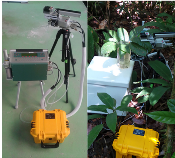
Fig. 1. Schematic image of LI6400XT and Less-P coupled system.
