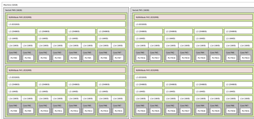
Figure 6.8: Topology of a ccNUMA Bulldozer server using hwloc.
