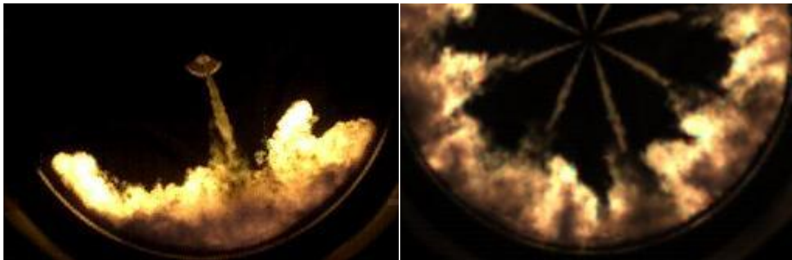
Figure 1.6: One combustion flame compared to eight combustion flames at 1500 bar injection pressure. This image is derived from the licentiate thesis of Dembinski H. W. R. [17].
