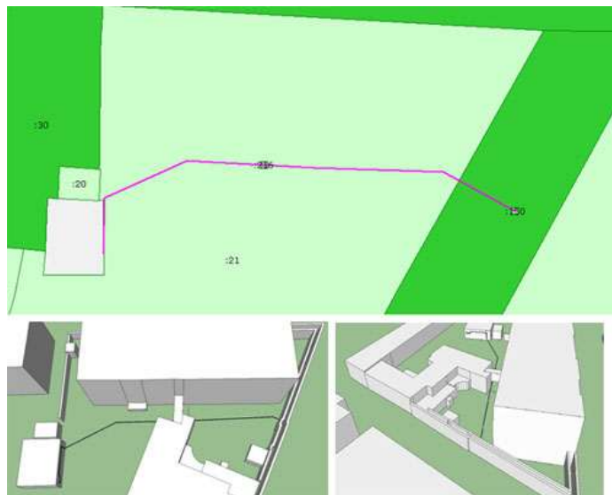
Figure 4.1: At the top the cadastral map fragment including the pipeline and at the bottom two different 3D views are depicted [Van Oosterom et al., 2012].
