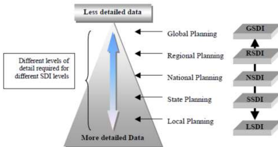
Figure 3.9: Relationship between spatial data and the different level of SDIs [Rajabifard et al., 1999].
