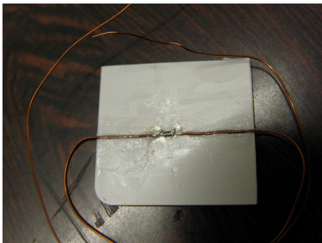
Figure 5.11: The sample is between the two wires and conductive contact was established with the use of conductive paint at the edges of the sample where the wires were glued.
