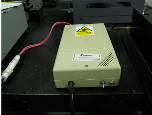
Figure 5.12: DC power supply which provides the high voltage to our apparatus.
