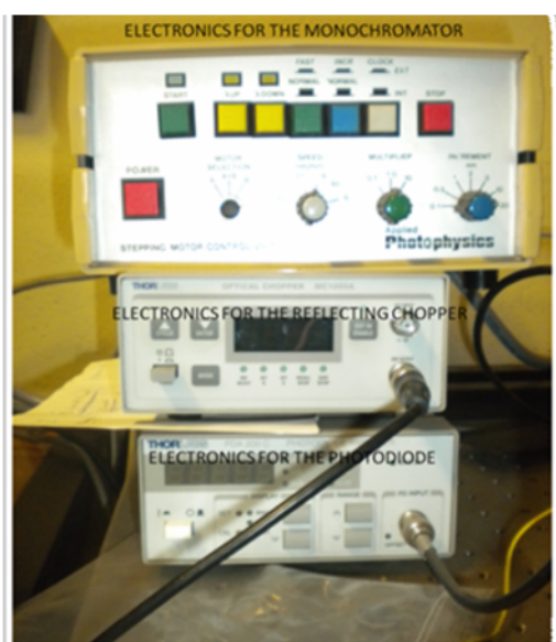
Figure 4.1.4 the electronics of the monochromator, the aluminum chopper, and the photodiode detector
