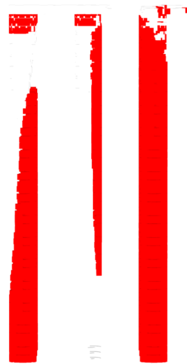
Figure 5.17. Pile-group plastic points i.e. the plasticized Mohr – Coulomb points (red) and the tension cut-off points (white)
