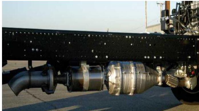
Figure 13: Particulate filter of HDD engine
