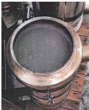
Figure 24: The two DCL particulate filters (26)
