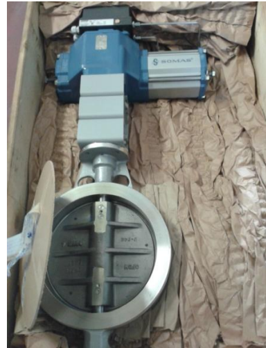
Figure 63: Butterfly valves as delivered in LME
