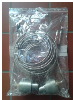
Figure 33: Lenses with fibre optic cables
