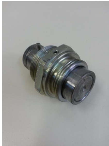
Figure 93: Flow meter adaptor for the second measuring position
