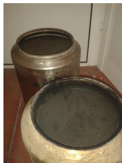
Figure 65: The two DPFs collected before their installation
