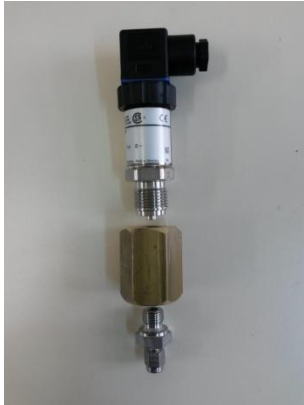
Figure 85: Pressure sensor - union - Parker adaptor
