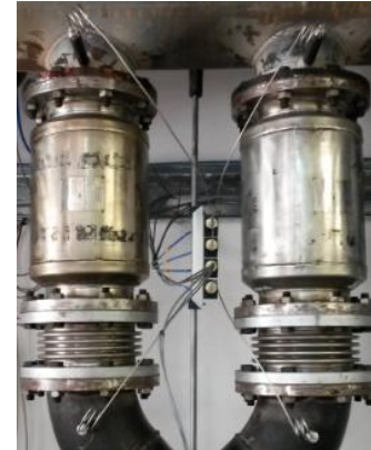
Figure 87: Pressure sensors process connection
