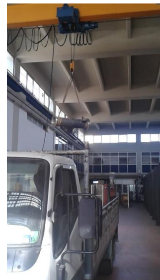
Figure 59: Parts transfer with the overhead crane
