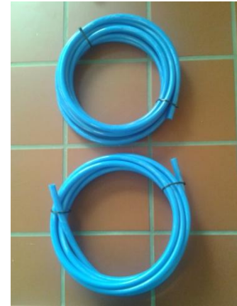
Figure 38: Air hoses of purge air system
