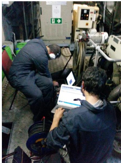
Figure 114: Portable DAQ system
