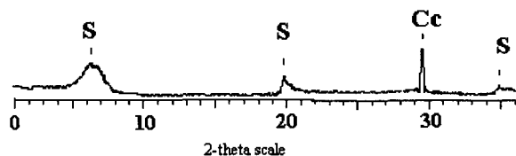
Figure 2. X-ray diffraction pattern of Milos-Island Na-activated bentonite. S = Smectite, Cc = Calcite.
