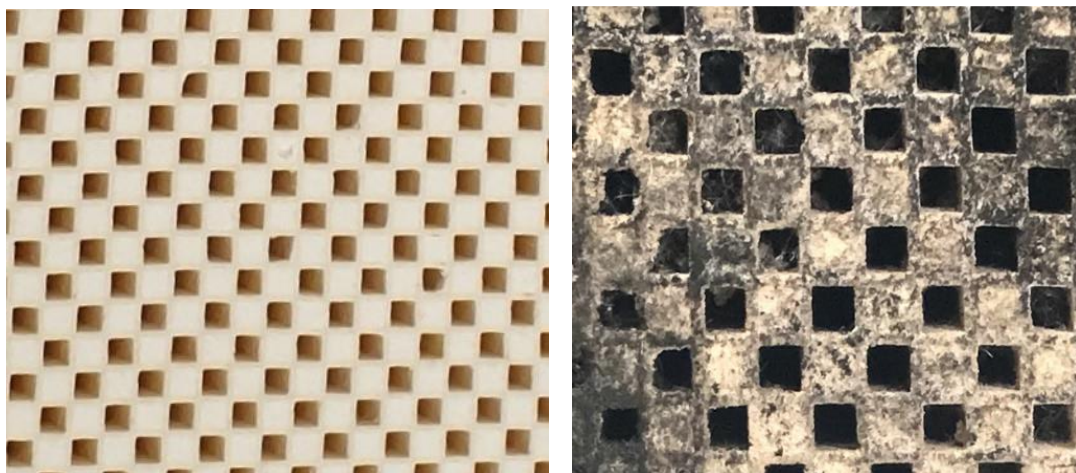
Figure 3.10 - DPF channel structure and condition before experimentation (left) and after experimentation (right)
