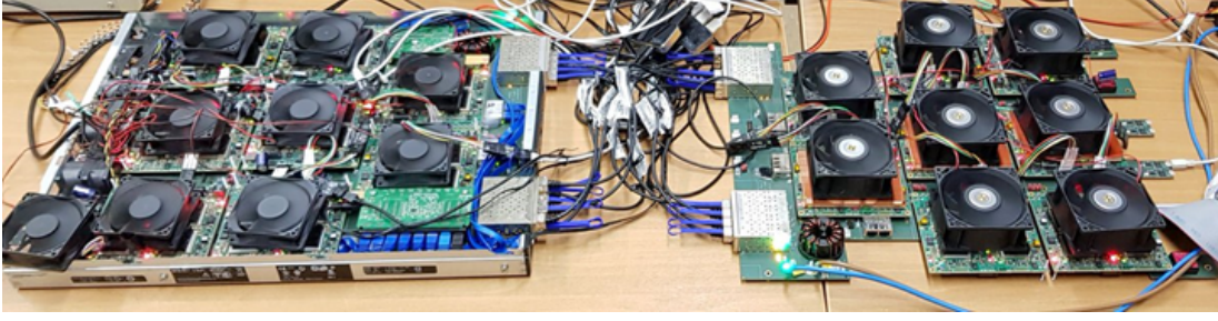
Figure 6.8: The ECOSCALE platform with 16 QFDBs (64 FPGAs and 1TB RAM) is used in this case study.
