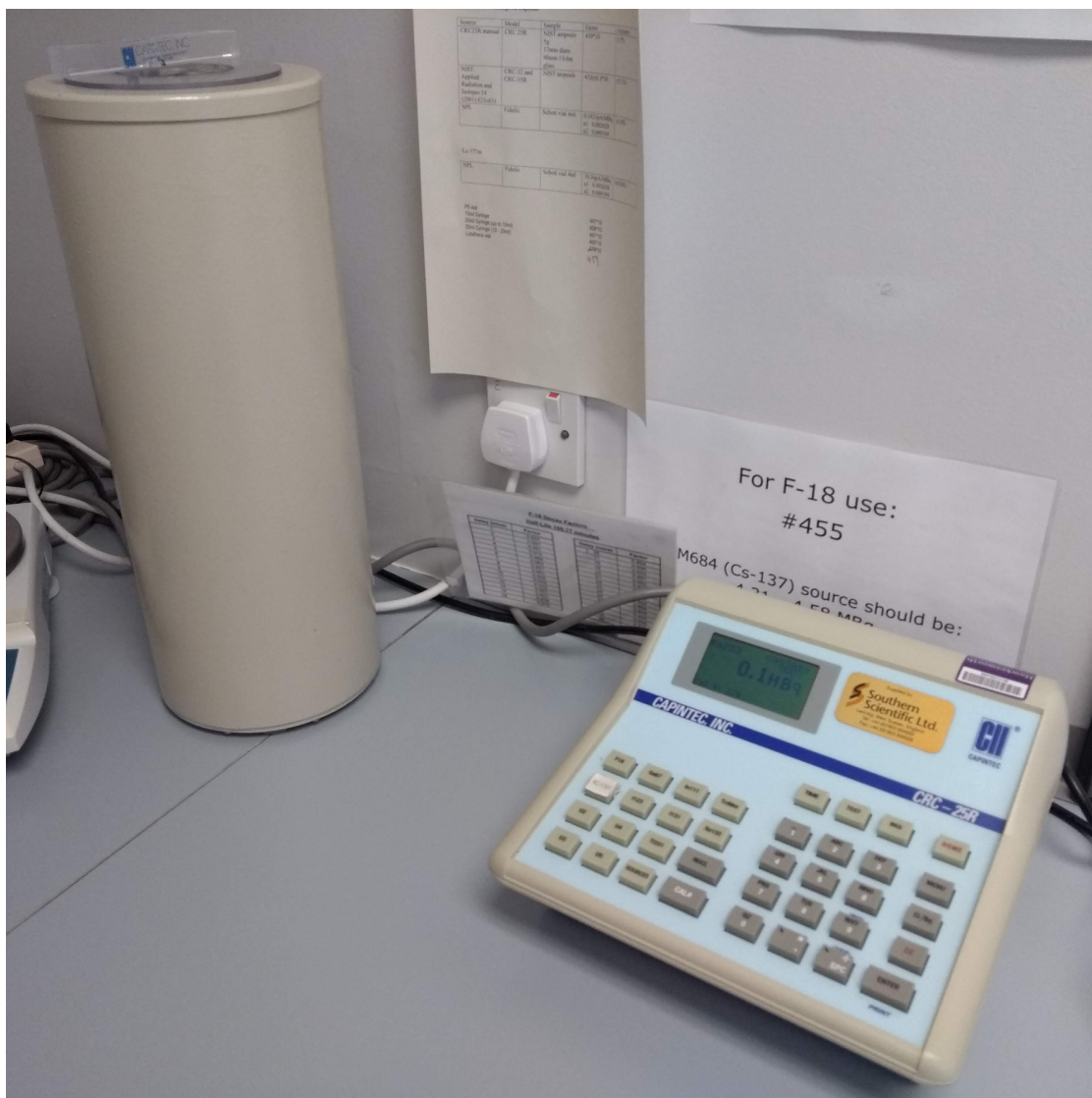
FIGURE 2.16: A photograph of a radionuclide calibrator at the Christie Hospital. On the left is the ionisation chamber detector into which samples are placed. On the right is the digital readout display. This figure is taken from reference [14].
