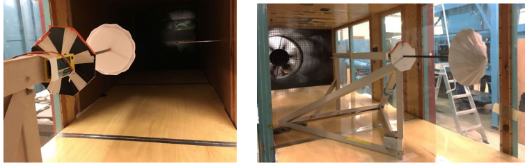
Figure 5: The wind tunnel setup, with a paper origami model mounted on a free-spinning axle that spins with a code disk used for spin rate measurement.
