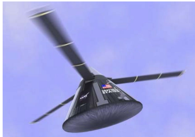
Figure 1.10: NASA Mars crewed vehicle concept equipped with a free-spinning foldable rotary wing decelerator that deploys at subsonic speed and stratosphere altitude, to enable precise landing manoeuvres [91]
