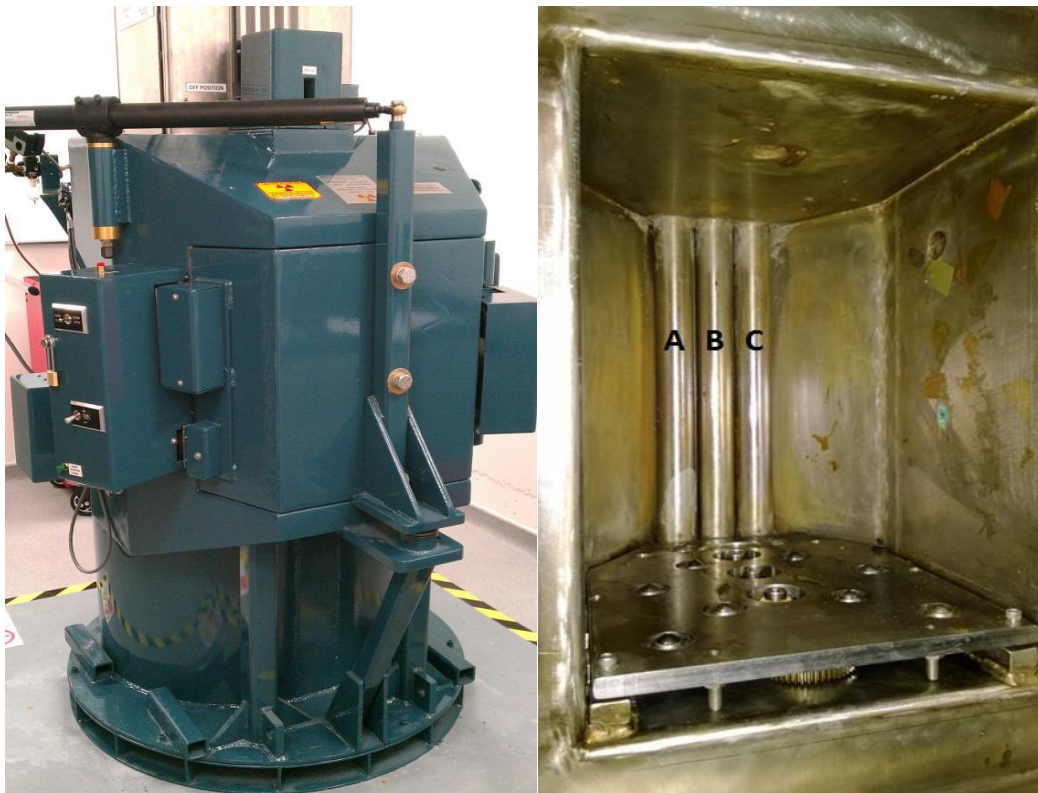
Figure 5.1-7. The image on the right shows the inside of the Foss therapy irradiator, with the labelled components showing the position of the three guided rods that contain the ^{60}\text{Co} source that are utilised during irradiations
