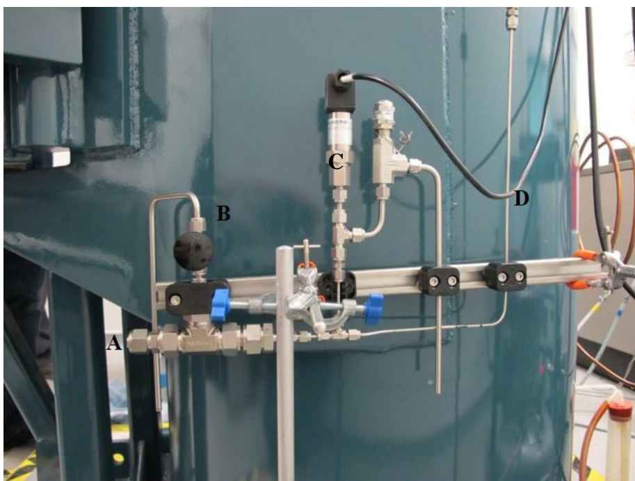
Figure 6.2-9. Photograph to show the reference electrode set up used in the recirculation loop system.
