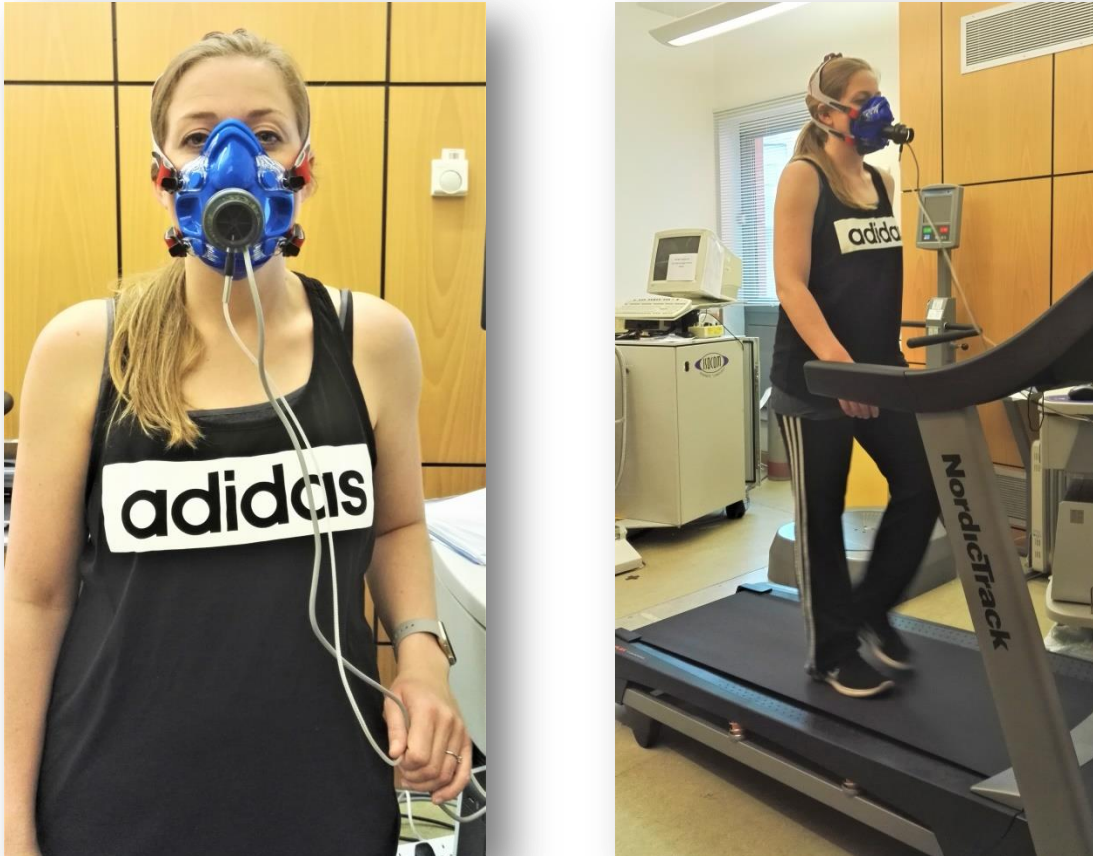
Figure 3.1 – Laura Smith demonstrating set up and procedure for cardiopulmonary exercise testing procedure. Clockwise from top left: Participants were fitted with a silicone face mask according to face size with head cap. Flowmeter with sampling lead was then connected to face mask. Participants began the exercise testing procedure after warm up period. During the testing procedure pulse rate and breath-by-breath gas exchange analysis was monitored. Treadmill gradient and incline was altered manually during the testing procedure. Courtesy of Laura Smith
