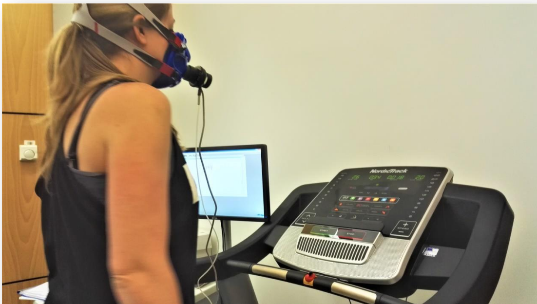
Figure 3.1 – Laura Smith demonstrating set up and procedure for cardiopulmonary exercise testing procedure. Clockwise from top left: Participants were fitted with a silicone face mask according to face size with head cap. Flowmeter with sampling lead was then connected to face mask. Participants began the exercise testing procedure after warm up period. During the testing procedure pulse rate and breath-by-breath gas exchange analysis was monitored. Treadmill gradient and incline was altered manually during the testing procedure. Courtesy of Laura Smith
