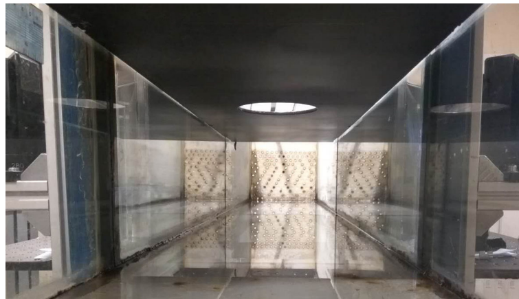
Figure 3.3: Front view of the flat plate test surface in the laminar boundary layer. The disc plate is not installed in the D = 132\text{mm} hole.
