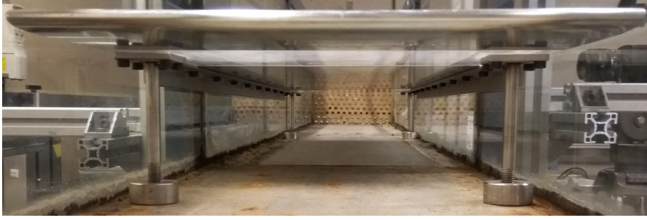
Figure 3.13: Front view of the leading edge and supporting thread legs of the flat plate. The test section of the plate is on the upper side and not shown here.
