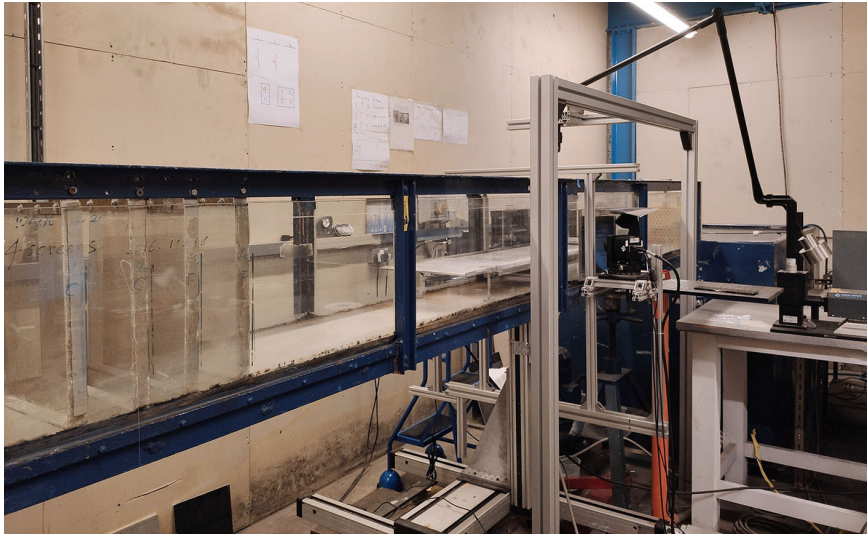
Figure 3.1: Perspective view of the experimental facilities. The setting shown is for stereoscopic PIV measurements in the boundary layer.
