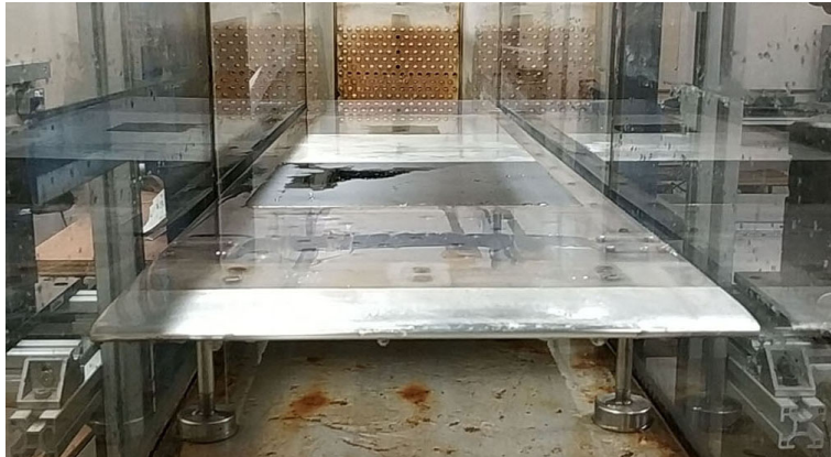
Figure 3.4: Front view of the flat plate test surface in the turbulent boundary layer. The cavity is filled with tiles having smooth surfaces.
