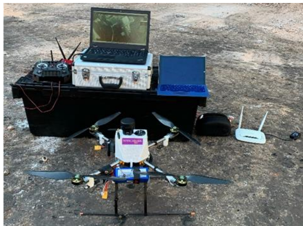
Figure 2: Aerial mapping system for stockpile volume estimation in cement plants including quadrotor with integrated sensors and ground station.
