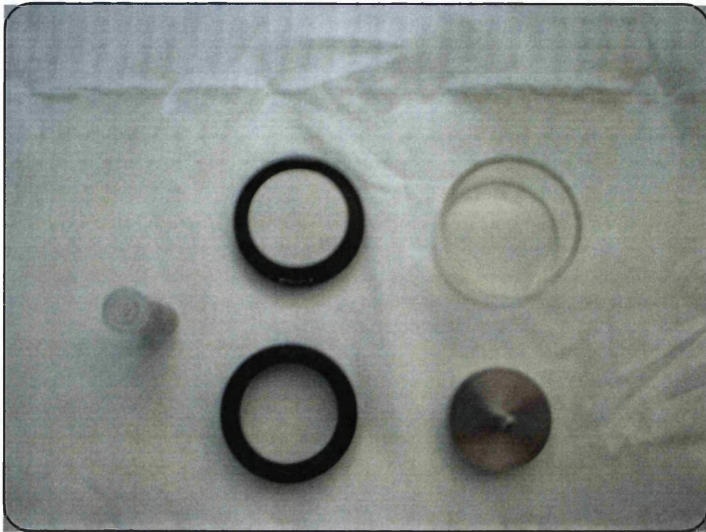
Figure 3.3.1 Sample Presentation Accessories Viewed from Above (HPLC glass vial, agricultural cell and reflectance vessel with stainless steel disc)
