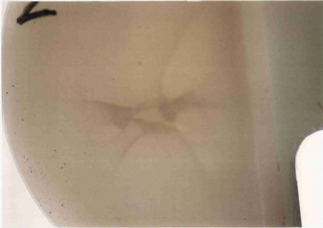
Figure 7.7 Photograph of the delaminated Kinematic (test one)
