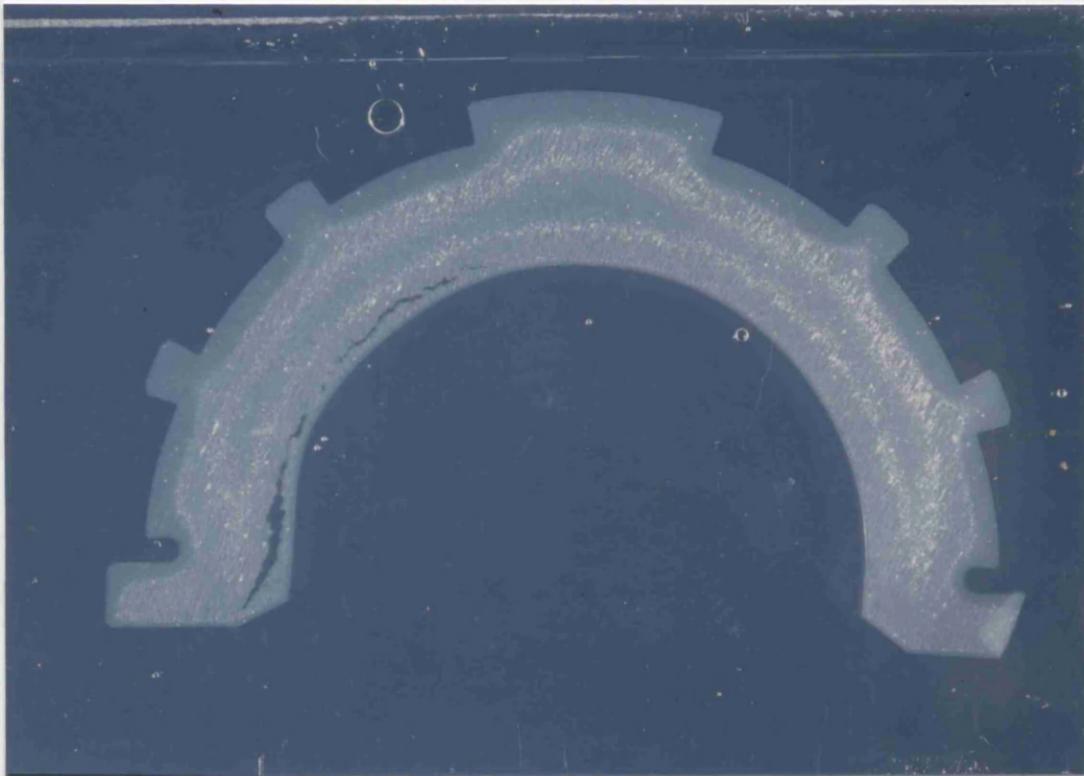
Figure 7.2b Thin section through a twelve year shelf-aged extruded component, showing a sub-surface 'white band'
