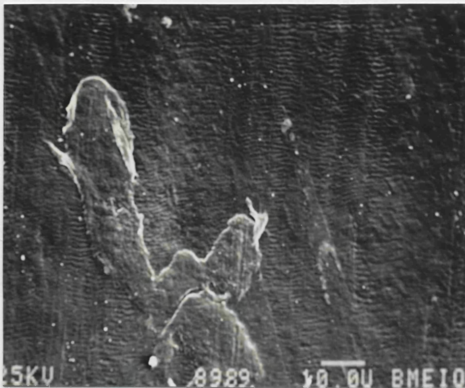
Figure 6.9 Scanning electron micrograph showing the ripple pattern on the stabilised polyethylene surface and sheets of polyethylene
