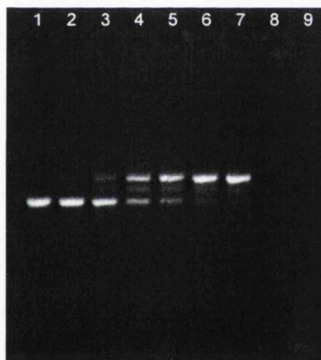
Figure 14 Gel showing the co-amplification of IS(B)3 and pHKY531 to generate a calibration curve. Where the pHKY531 concentration (molecules 10 \mu\text{L}^{-1} ) was:
