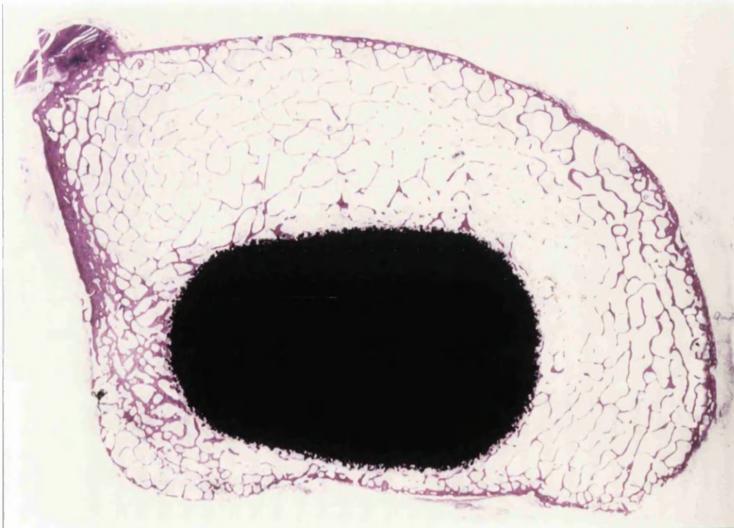
Figure 14: A thin section through a plain porous specimen showing increased bone growth in the medial aspect.
