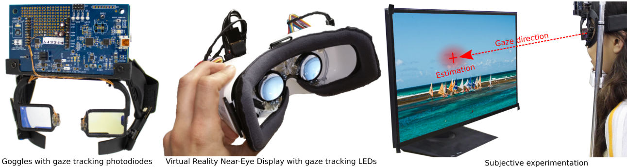
Goggles with gaze tracking photodiodes
