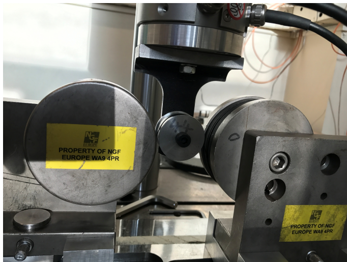
Figure 1: Testing setup for tension-bending coupling fatigue loading.
