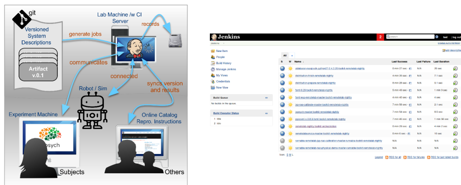
Figure 10.2: Toolchain for the replication of robotics experiments: An experiment for which the associated computational artifacts are documented in a browsable online catalog which is linked to the corresponding repositories. From here a researcher is instructed to automatically roll out the system distribution using a continuous integration server which is linked to the robot platform as well as the computer controlling the behavioral experiment using JsPsych. Left: Overview of the toolchain, Right: Screenshot of the CI server web front-end. Each row corresponds to a recipe that has been translated into a build job. Build jobs can be activated by selecting the most right icon (stopwatch). Execution of an experiment can also be triggered using this front-end.
