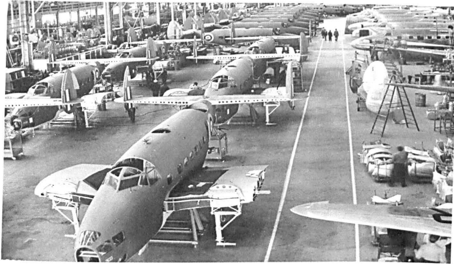
1. The production line of Hudsons of the Lockheed Corporation's Works at Burbank. They fulfilled their contracts on time, and maintained liaison with No 224 Squadron.
