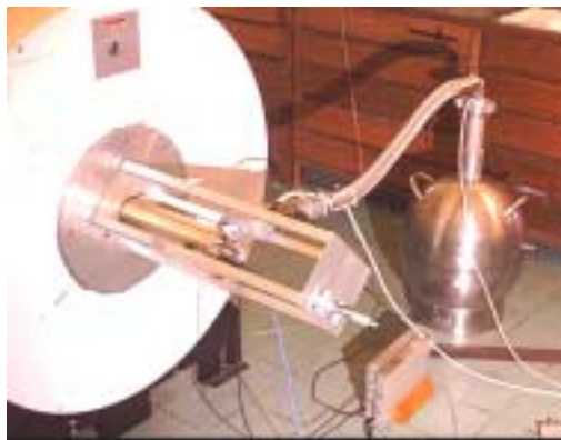
Figure 20: Gas flow cooling system, shown with 3D imaging system in the stray field configuration.
