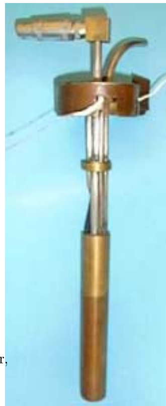
Figure 17: Liquid nitrogen cooled cryoporometry NMR probe, used for bulk and 1D measurements.
