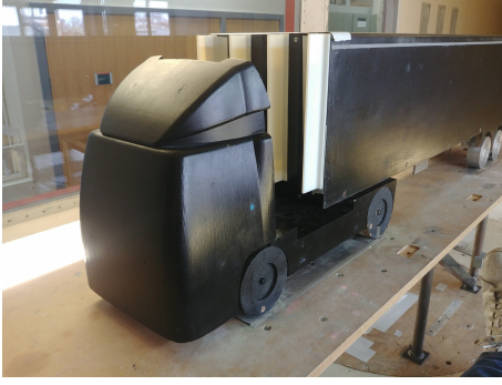
Figure 6: 1:10 th scale model with four CVTDs attached to the trailer front face
