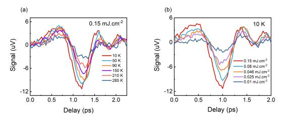
Figure H.1: Time domain data of THz emission from YIG/Pt for varying (a) temperature at  $0.15 \text{ mJ/cm}^2$  and (b) pump fluence at a constant temperature 10 K
