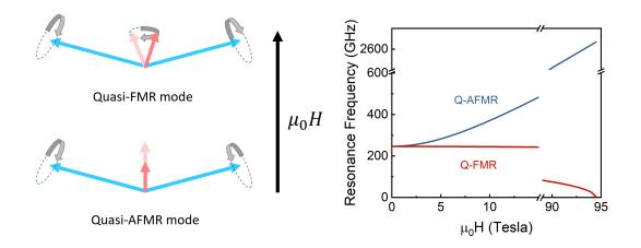
Figure 2.7: (left) Antiferromagnetic resonance modes when the external is applied perpendicular with the antiferromagnetic axis, resulting a quasi-FMR mode where the net moment precesses, or quasi-AFMR mode where the magnitude of the net moment oscillates, and (right) the corresponding frequency dependence of the field
