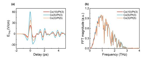
Figure F.2: A comparison between THz emitted from the Co(10)/Pt(3), Co(5)/Pt(3)and Co(3)/Pt(5), pumped with 25  $\mu$ J energy per pulse using the Galilean telescope in (a) time domain (b) frequency domain
