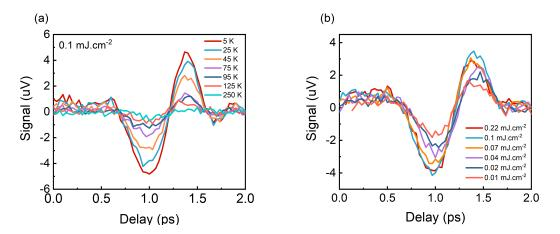
Figure I.1: Time domain data of THz emission from  $KNiF_3/Pt$  for varying (a) temperature at 0.15 mJ/cm<sup>2</sup> and (b) pump fluence at a constant temperature 10 K
