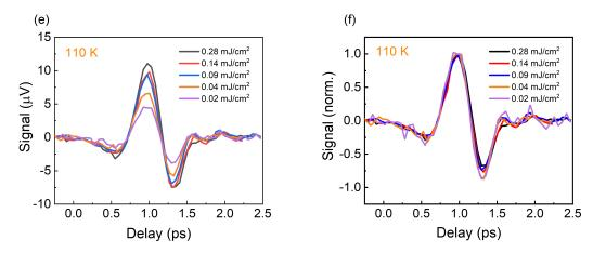
Figure J.3: (a) Raw and (b) normalised time domain data of THz emission from  $KCoF_3/Pt$  for varying pump fluence at 110 K
