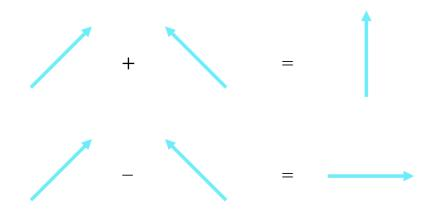
Figure 3.7: Illustration polarisation-resolved THz measurements, performed by acquiring THz signals when  $1^{st}$  wire grid polariser is  $+45^{o}$  and  $-45^{o}$  to the  $2^{nd}$  polariser. The blue arrows represent  $E_{THz}$  polarisation after the  $1^{st}$  wire-grid polariser. Summation gives a THz polarisation along the  $2^{nd}$  polariser, which is vertical, while subtraction gives the perpendicular component
