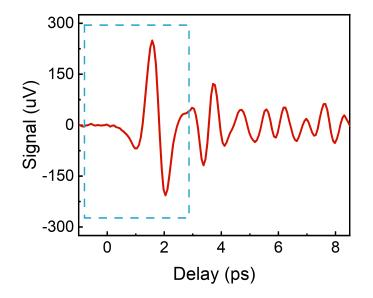
Figure B.1: The first THz time-domain data from our setup. The blue dashed rectangle indicates the actual signal from the ZnTe emitter
