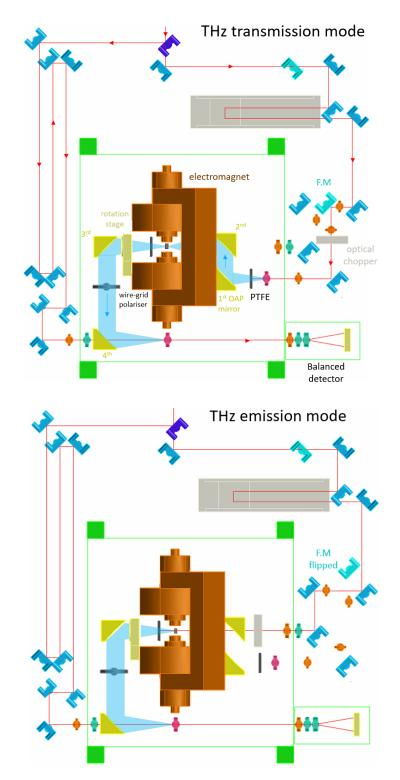
Figure 3.3: Beam trajectory in (top) THz transmission mode and (bottom) THz emission mode where flipping a mirror and a lens and moving the optical chopper are required
