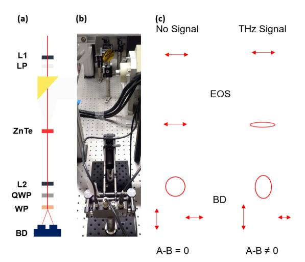
Figure 3.5: (a) Schematic illustration and (b) photograph of the electro-optic sampling + balanced detection assembly, (c) illustrations of balanced detection in detecting phase change in the probe beam
