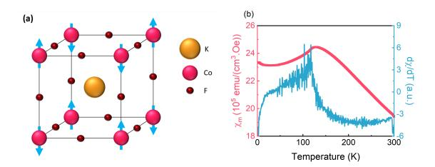
Figure 6.1: (a) Illustration of  $\text{KCoF}_3$  crystal structure (b) SQUID measurement of magnetic moment (0.1 Tesla field applied) as a function of temperature, showing a peak at 117 K
