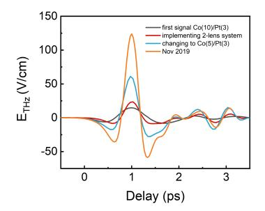
Figure 3.9: THz emission signal enhancements: (black) the first signal, (red) implementing a 2-lens system for larger beam diameter, (blue) changing Co/Pt calibration sample, and (orange) fine alignment procedures until November 2019
