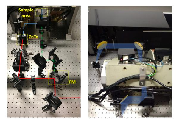
Figure 3.4: (a) Pump beam steering in THz transmission or THz emission setup (b) THz beam steering using 4 off-axis parabolic mirrors
