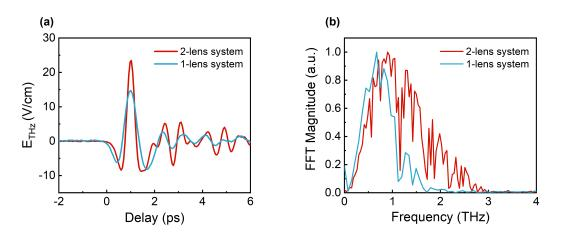
Figure F.1: A comparison between Co(10)/Pt(3) THz emission using (a) the onelens system and (b) the two-lens system
