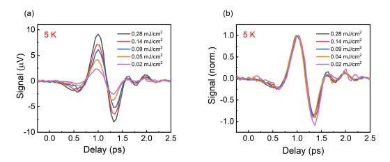
Figure J.1: (a) Raw and (b) normalised time domain data of THz emission from  $KCoF_3/Pt$  for varying pump fluence at 5 K
