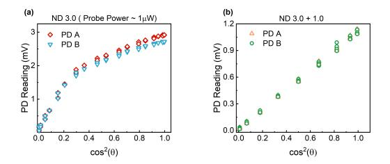
Figure B.6: Monitor reading dependence on  $\cos^2(\theta)$  of angle between probe polarisation and the polariser axis. It should be linear as expected from Malus' Law. The two figures use different maximum probe power controlled by ND filters (a) ND 3.0 (b) ND 3.0 + 1.0
