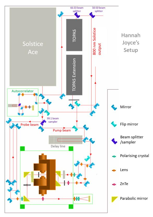
Figure 3.1: Illustration of the THz setup
