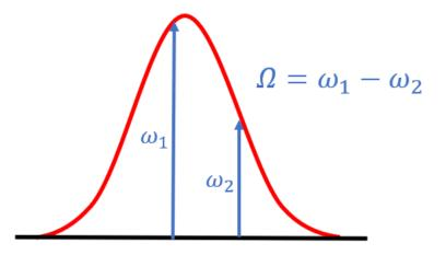
Figure 2.1: An illustration of difference frequency generation within a femtosecond pulse which results in a broadband Terahertz pulse
