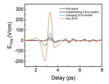
Figure 3.8: THz transmission signal enhancements: (black) the first signal, (red) implementing a 3-lens system for larger beam diameter, (blue) changing the ZnTe emitter crystal, and (orange) fine alignment procedures until November 2019
