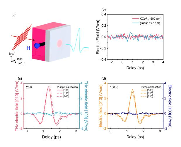
Figure 6.4: (a) Illustration of THz emission experiments in  $\text{KCoF}_3/\text{Pt}$  (b) Control measurements using a bulk  $\text{KCoF}_3$  (pink) and glass/Pt(7nm) (light blue) which both show no signal (c) Time-domain trace of polarisation resolved THz emission  $(E_{THz}||[010]]$  and  $E_{THz}||[100])$  from  $\text{KCoF}_3/\text{Pt}$  at 20 K and (d) at 150 K
