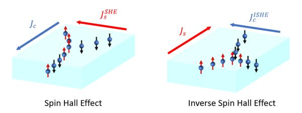
Figure 2.5: A schematic illustration of spin Hall effects where spin-dependent scatterings induce a transverse pure spin current, as well as the inverse spin Hall effect
