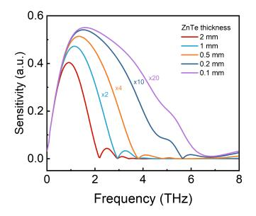
Figure 3.6: Calculated frequency spectrum of electro-optic sampling using ZnTe 1  $\rm mm$
