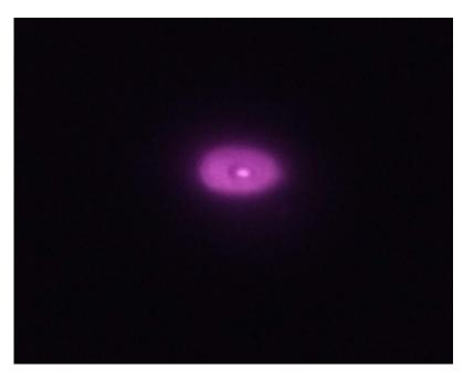
Figure A.1: A picture of spatial overlap between the probe beam (smaller stronger spot at the centre) and the THz beam, which is represented by 800 nm light surrounding the probe beam
