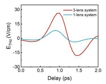
Figure C.2: THz peak obtained with three-lens system compared to one-lens system
