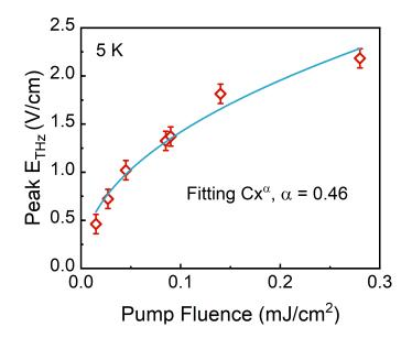
Figure 4.8: Peak PSSE signal dependence on pump fluence at 5 K. The fitting originates from  $\Delta T_e \sim const. U_{abs}^{0.5}$  for low sample temperatures
