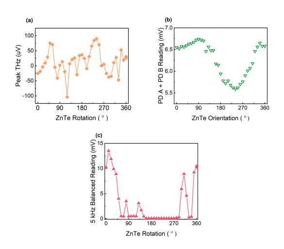
Figure B.3: The influence of ZnTe detector orientation on (a) Peak time-domain THz signal, (b) total probe intensity read by the two photodiodes, (c) minimized 5 kHz balanced channel output
