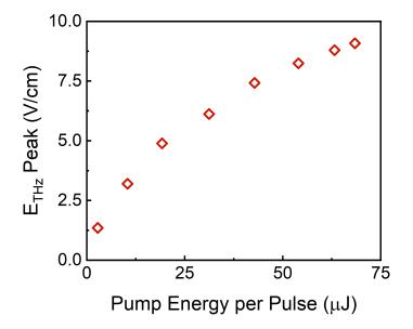
Figure B.7: THz electric field peak (V/cm) as a function of pump energy per pulse
