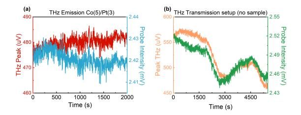
Figure 3.11: Signal stability of THz emission setup (a) in normal circumstances and (b) when the ambient temperature fluctuates
