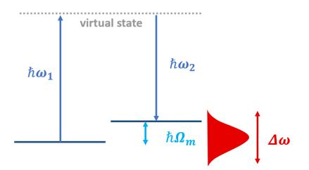
Figure 2.4: A schematic illustration of impulsive stimulated Raman scattering, where an inelastic scattering assisted by a virtual state can induce modes in THz frequencies. If the two ground states have different spin state, the scattering excites a magnon
