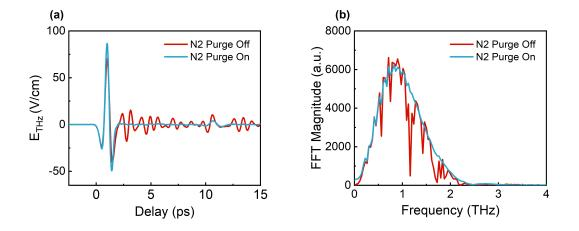
Figure 3.10: (a) Time domain and (b) frequency domain of THz emission with (blue line) and without (red line)  $N_2$  purging
