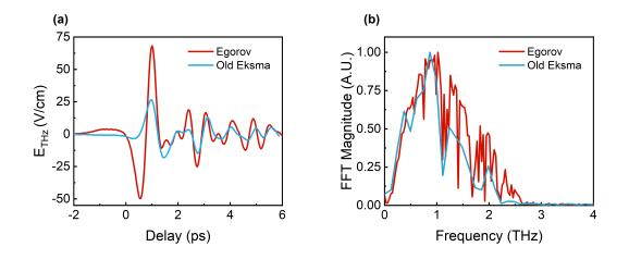
Figure D.1: (a) Time-domain (b) frequency domain data of THz emitted by the ZnTe crystal from Egorov Scientific
