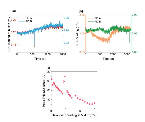
Figure B.5: Probe stability as read by the two monitor channels: (a) the desired signals (b) when the readings change over time. (c) Peak THz signal at 2.5 kHz as a function of balanced channel reading at 5 kHz
