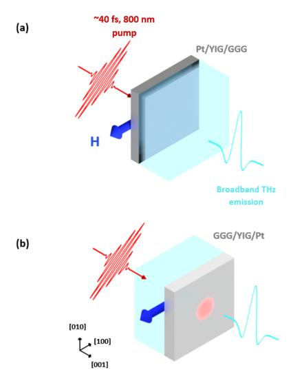
Figure 4.3: Illustration of the THz emission experiment using 40 fs optical pulse with central wavelength of  $\omega = 800$  nm. The ultrafast build-up of the interfacial temperature difference injects pure spin current, which is converted to THz charge current by the ISHE. Two configurations used in the experiment (a) GGG substrateside pumping (b) Pt-side pumping
