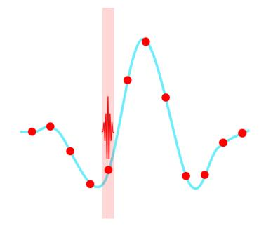
Figure 2.2: An illustration using electro-optic sampling to map a time-domain profile of a THz pulse (blue) by acquiring reading at different time delays with a optical probe pulse (red bullets)
