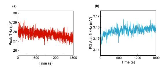
Figure B.4: (a) Peak THz pulse signal stability and (b) the corresponding monitor reading of 1st version of the setup
