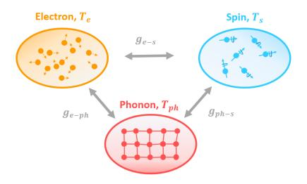
Figure 2.3: An illustration of three temperature model which treats electrons, spins, and phonons as separate systems with an internal temperature
