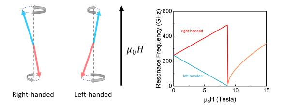
Figure 2.6: (left) an illustration of two easy-axis antiferromagnets in anti-parallel resonance modes with two opposing chirality and (right) the corresponding frequencies as function of applied external field. For a strong field  $H_{SF} = \sqrt{2H_EH_a}$ , the exchange and the anisotropy energy is overcome and the two sublattices undergo a 90<sup>o</sup> rotation
