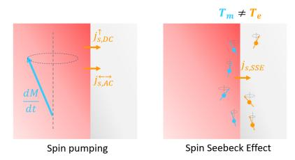
Figure 2.8: An illustration of (left) spin pumping and (right) spin Seebeck effect, where the former refers to a coherent precessional motion of collective spins inducing a net spin transfer across the interface while the latter can be considered as the incoherent counterpart which is induced by thermal fluctuations
