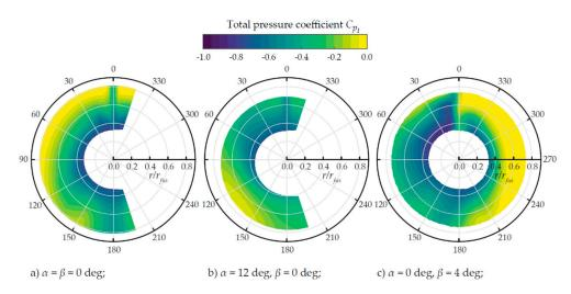
**Figure 16.** Total pressure field upstream of the FF air intake ( $x/L_{fus} = 0.89$ ) in cruise and off-design conditions. Measurements taken on the 3D PFC setup at  $V_0 = 40$  m/s.
