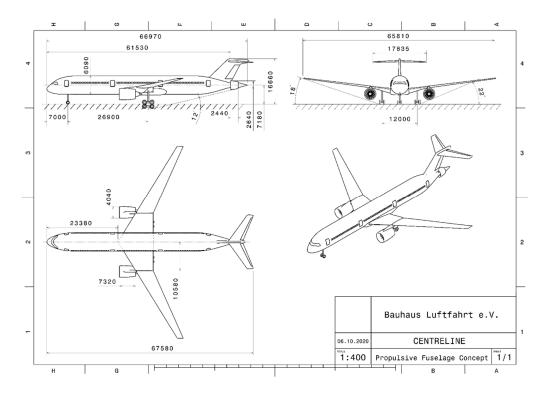
Figure 34. Three-view of the baseline member of the CENTRELINE PFC aircraft family, dimensions in mm.
