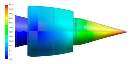
**Figure 25.** Displacement map for aft-fuselage nacelle and integration structure of PFC Rev07 design case 2 under CS 25.561 loads. Color legend shows vertical displacement in mm.
