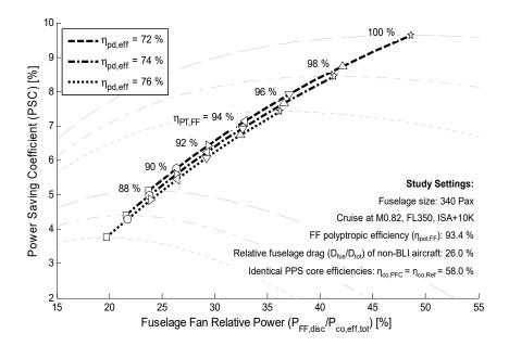
**Figure 32.** Identification of optimum power savings and corresponding FF cruise power settings for combinations of power train and non-BLI propulsive device efficiencies.
