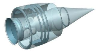
Figure 22. Basic visualization of CENTRELINE aft-fuselage aero-structural integration concept.
