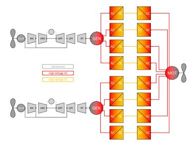
Figure 26. Overall propulsion system architecture (Source [81]).
