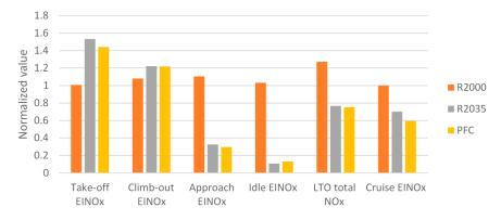
Figure 38. NO<sub>x</sub> emissions assessments results for the CENTRELINE R2000, R2035 & PFC aircraft.
