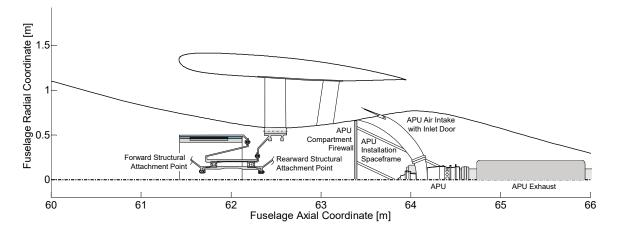
Figure 20. Concept sketch of the aft-fuselage power plant integration.
