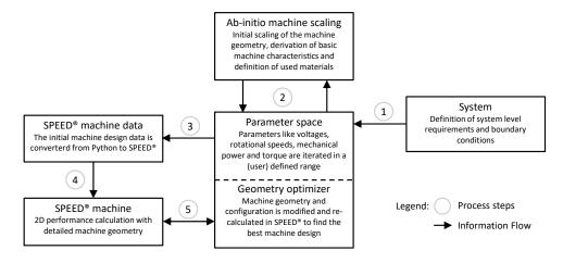
Figure 27. Basic electric machine design scheme.
