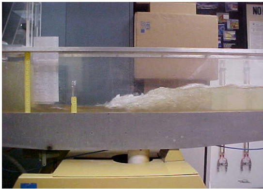
Figure 3. Calculate Hydraulic Jump Length
