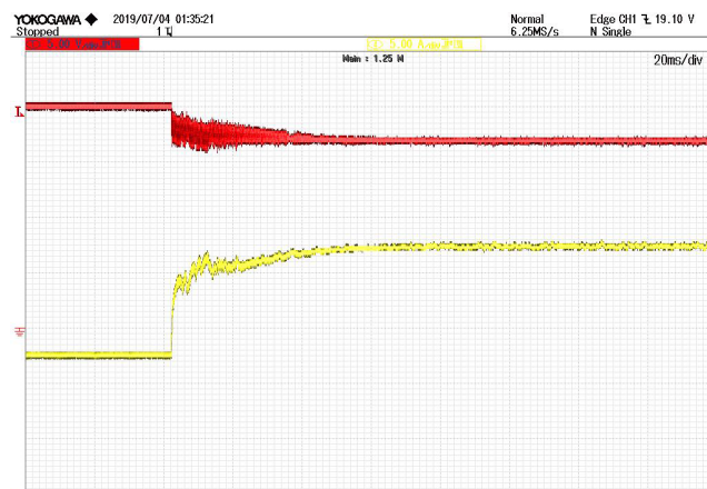
Fig. 14. System response to a step from P = 250 W to P = 380 W with the controlled shunt damper. Red curve (top) corresponds to the voltage x_2 (5 V/div) and yellow curve (bottom) corresponds to the current x_1 (5 A/div). Time scale is 20 ms/div.
