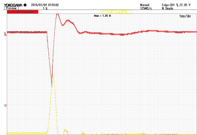
Fig. 13. System response to a step from P = 10 W to P = 300 W without the controlled shunt damper. Red curve (top) corresponds to the voltage x_2 (5 V/div) and yellow curve (bottom) corresponds to the current x_1 (5 A/div). Time scale is 1 ms/div.
