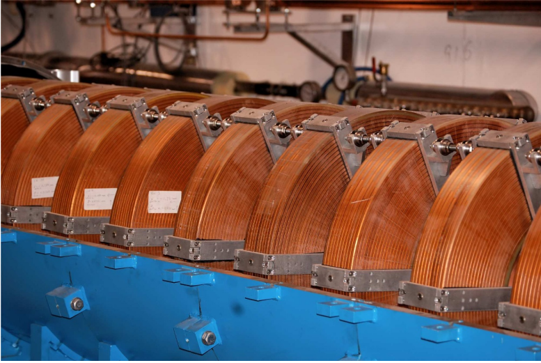
Fig. 12.3. Solenoid coils embedding the first accelerating S-band structure; the upper iron shield is removed.
