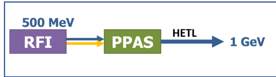
Fig. 23.40. Scheme 5 combining a 500 MeV RF injector with a PPAS to 1 GeV.
