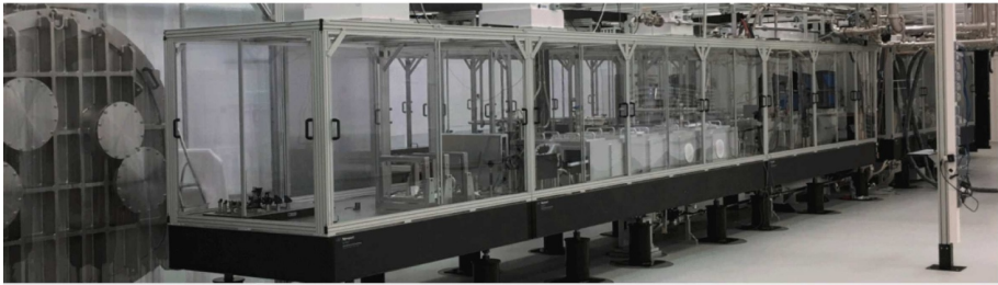
Fig. 29.8. The L3 “HAPLS” laser system at ELI-Beamlines (30 J, 10 Hz) (image courtesy of ELI Beamlines).
