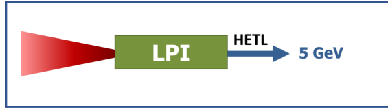
Fig. 23.4. Scheme 1 using a single-stage injector / accelerator generating an FEL-quality 5 GeV beam.
