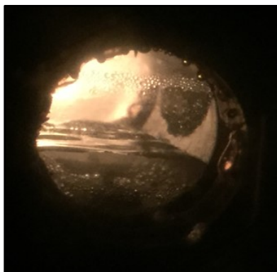
Figure 6.18: Formation of isobutene by an acidic catalysed dehydration of tert -butanol.
