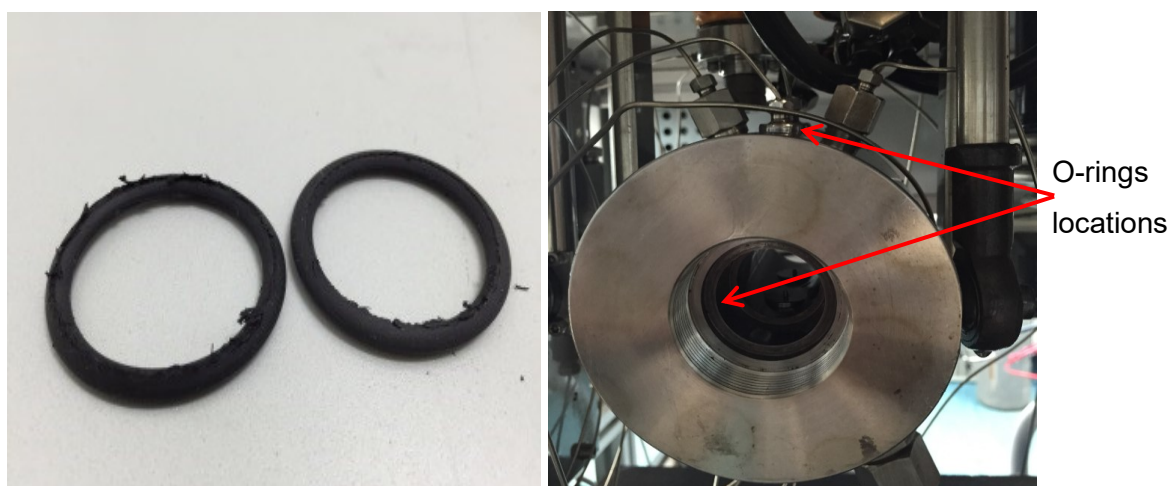
Figure 4.7: Schematic of the O-rings in the VC. Left shows the damages, Right shows the locations of the sealing required in the VC.
