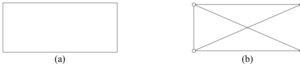
Figure 4.1: Basic units for modeling (a) continuum (Basic Continuum Unit - BCU) and (b) discrete structures (Basic Discrete Unit - BDU)
