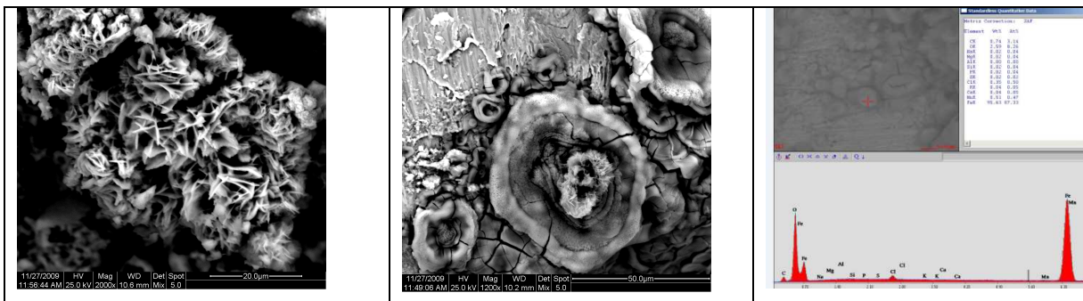
US1 after reduction for 18hrs by hydrogen plasma at low temperature
