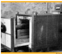
Fig. (4-4) Hydrogen reduction After: The Metals Conservation Summer Institute 2006
