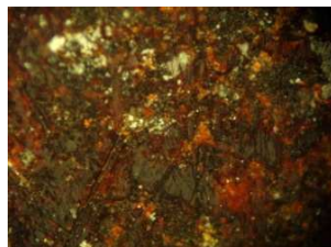
B1, After 4 months immersing in sodium hydroxide combined by plasma reduction
