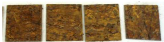
Photo (9-2) the coupons before the desalination treatment and after dividing for four parts
