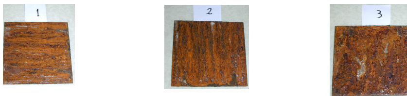
Photo (9-1) the iron coupons after accelerated aging and before dividing into four parts
