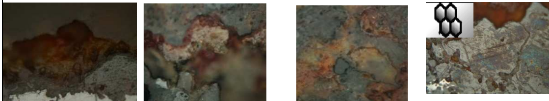
US8, The exterior layer of the marine compounds with the iron oxides. X500 US8, the intergranular corrosion X500
