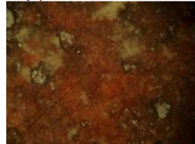
B3 after 24hrs reducing by hydrogen plasma followed by immersing in sodium hydroxide for 5 months. These photos are from the inside layer
