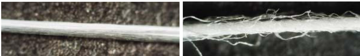
Figure 1-7: Flat yarn (left) and twisted multifilament yarn (right).
