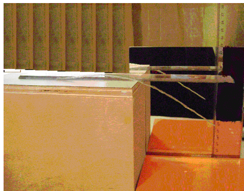
Figure 2-10: Yarn specimen subjected to bending test.
