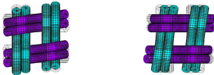
Figure 3-38: Deformed and undeformed shape of the basket unit cell in shear test (shear angle = 0.15) along warp (left) and weft direction (right).
