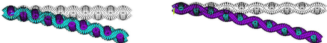
Figure 3-35: Deformed and undeformed shape of the plain woven model in bending test ( y/L = 0.2 ).
