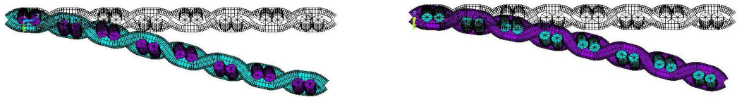
Figure 3-40: Deformed and undeformed shape of the basket model in bending test ( y/L = 0.2 ).
