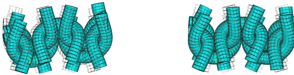
Figure 3-63: Deformed and undeformed shape of the interlock unit cell in shear test (shear angle = 0.15) along wale (left) and course direction (right).
