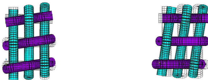
Figure 3-43: Deformed and undeformed shape of the twill unit cell in shear test (shear angle = 0.15) along warp (left) and weft direction (right).
