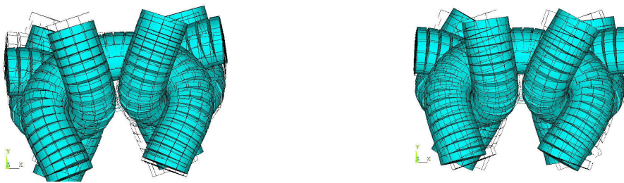
Figure 3-58: Deformed and undeformed shape of the rib 1 \times 1 unit cell in shear test (shear angle = 0.15) along wale (left) and course direction (right).
