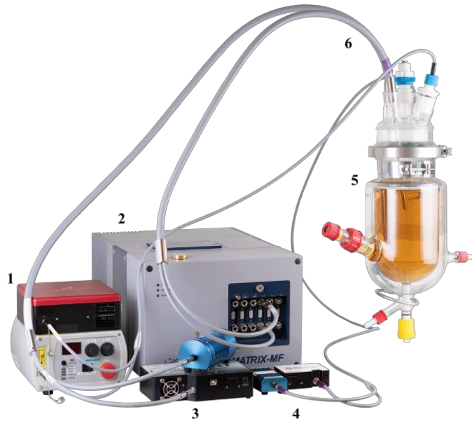
133 Fig. 1: Scheme of multispectral fiber system (figure courtesy of Art Photonics GmbH, Germany 134 [26]). Raman system (1); FTIR absorption System (2); NIR reflection System (3); fluorescence 135 detector (4); chemical reactor (5); and fiber optic probes (6).
