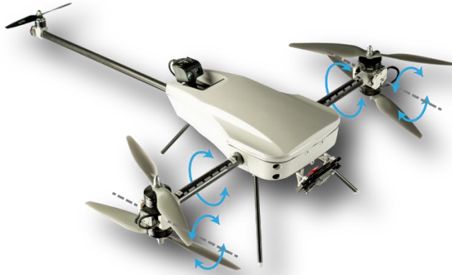
Fig. 1. The over-actuated Voliro multirotor UAV. Annotations show the additional degrees of freedom about which the main propeller pairs may be independently rotated.
