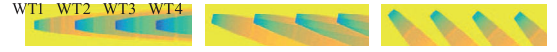
FIGURE 2 A 4-WT small example (wind direction is 0^\circ , 14^\circ , 45^\circ from left to right)
