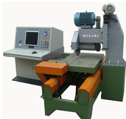
Fig. 2. The picture of diamond circular saw testing system
