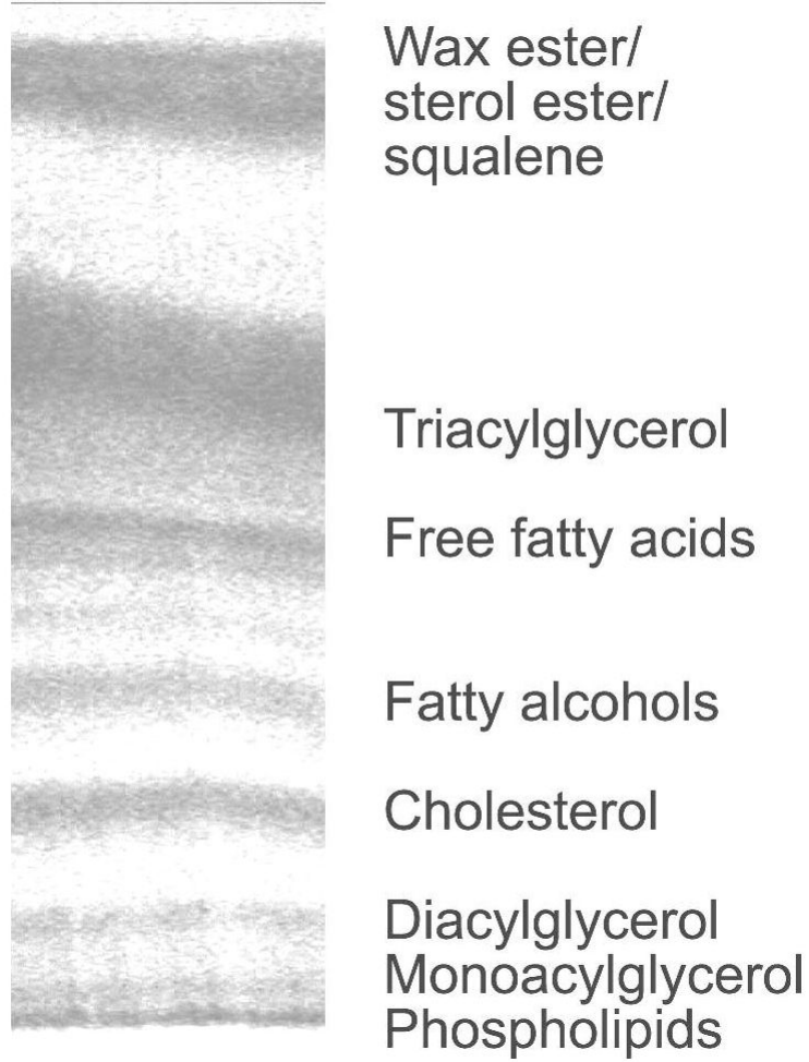
Figure 3. Separation of the lipid extract of vernix, using thin-layer chromatography. The separated lipid classes are indicated.
