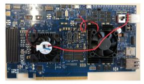
Figure 3: Shown is the novel PCIe ZYNQ MPSoC Data Aquisition Board developed at KIT.
