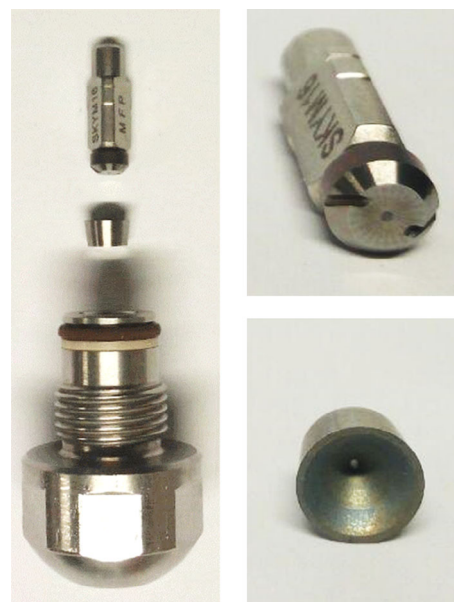
FIGURE 2 Pressure swirl nozzle SKHN-MFP. left: slotted core, orifice insert, and nozzle casing. up right: slotted core (front view). Down right: orifice insert (back view)
